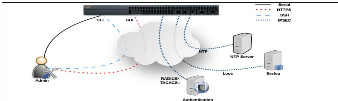
**Figure 1: TOE Architecture**
